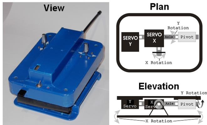
Fig. 1. View, plan and elevation of ungrounded haptic display used in Relay project.
