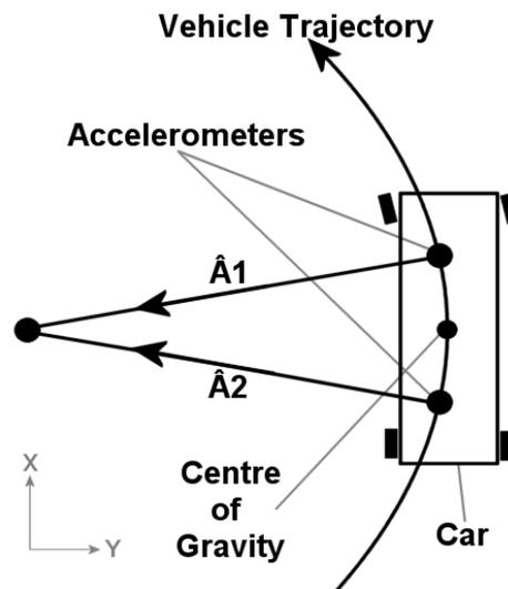
**Fig. 3.** Accelerations measured by two accelerometers mounted equidistant from the vehicle's center of gravity, supporting the measurement of slip.
